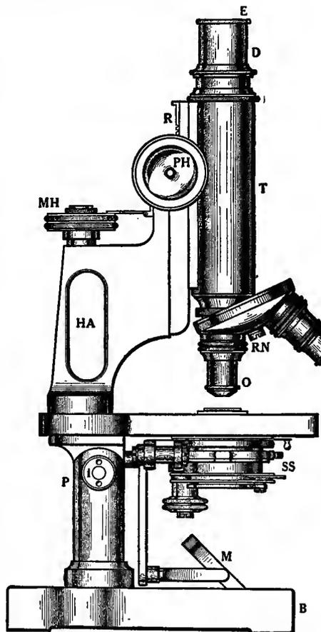
COMPOUND MICROSCOPE: E, Eyepiece; D, draw-tube; body-tube; RN, revolving nose-piece; O, objective PH, pinion head; MH, micrometer head; HA, hank arm; S, stage; SS, substage; M, mirror; B, base; rack; P, pillar; I, inclination joint.
