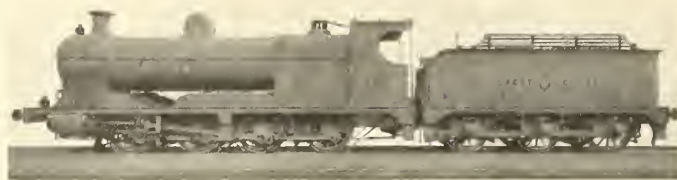
FIG. 442—J. G. ROBINSON'S EIGHT-COUPLED MINERAL ENGINE, GREAT CENTRAL RLY., 1902-10
