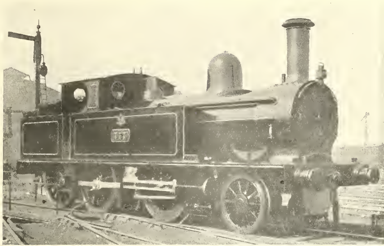
FIG. 314—L. & N.W.R. COMPOUND GOODS TANK ENGINE, 1887 (Photo. Locomotive)
