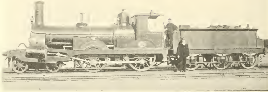
FIG. 256—D. JONES'S CONVERTED BOGIE ENGINE, HIGHLAND RAILWAY, 1873 [Photo, Locomotive]
