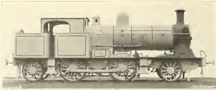
FIG. 388—BEYER, PEACOCK & CO.'S COMPOUND TANK ENGINE, BELFAST & COUNTY DOWN RLY., 1891
