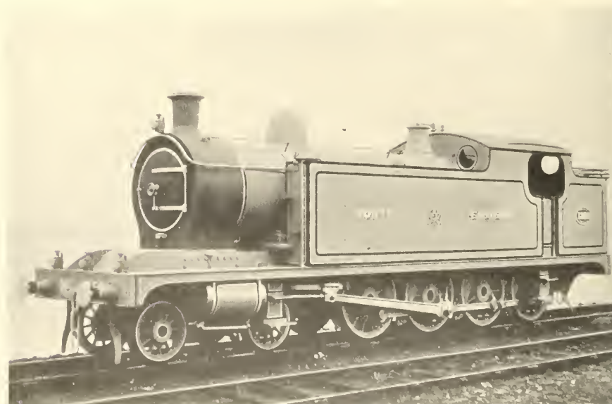
FIG. 427—W. WORSDELL'S THREE-CYLINDER SHUNTING TANK ENGINE, NORTH-EASTERN RLY., 1909
