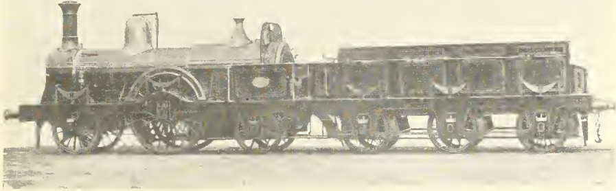
FIG. 183—CUDWORTH'S SINGLE DRIVER "MAIL" ENGINE, SOUTH EASTERN RLY., 1861
