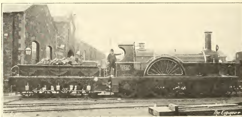
FIG. 271—G.W.R. BROAD GAUGE BOGIE EXPRESS ENGINE, 1877 [Photo. Locomotive]
