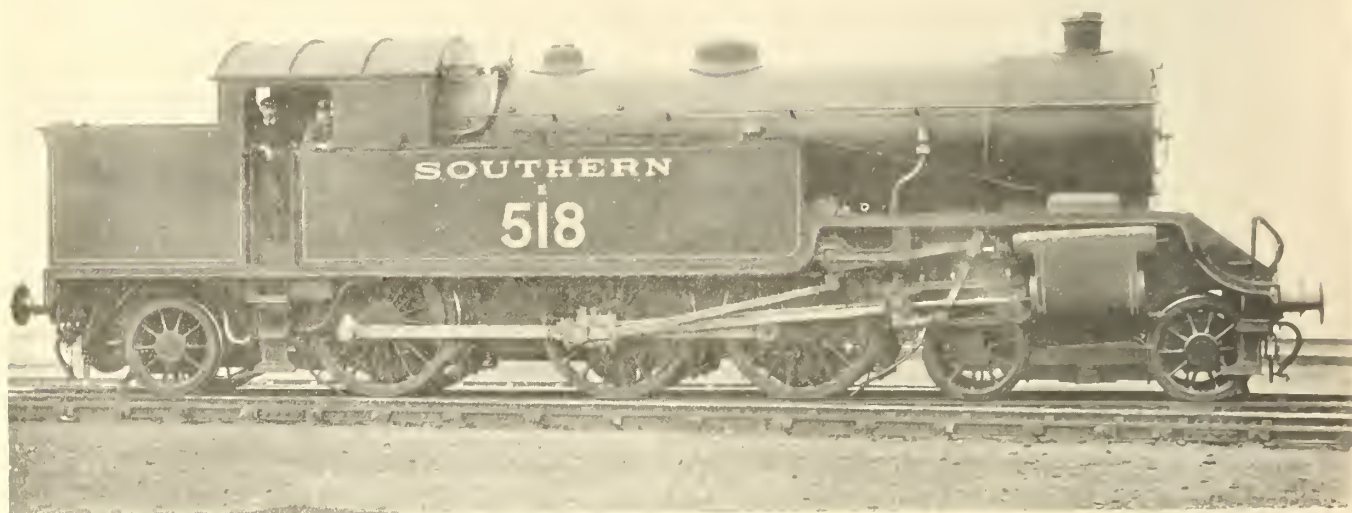
FIG. 464—R. W. URIE'S 4-6-2 GOODS TANK ENGINE, SOUTHERN RLY. (FORMERLY L. & S.W. RLY.), 1921
