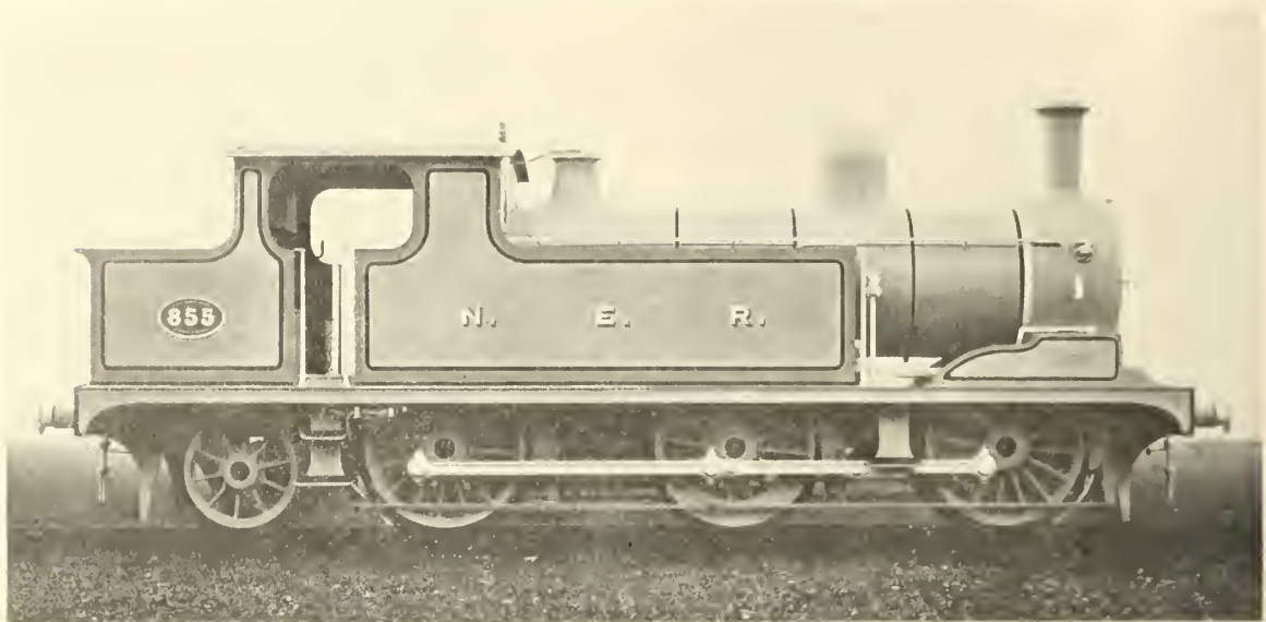
FIG. 320—T. W. WORSDELL'S COMPOUND GOODS TANK ENGINE, N.E.R., 1888
