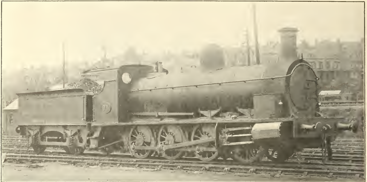
FIG. 356—SIARP. STEWART'S 8-COUPLED GOODS ENGINE, AS MODIFIED FOR THE BARRY RLY., 1889-97
