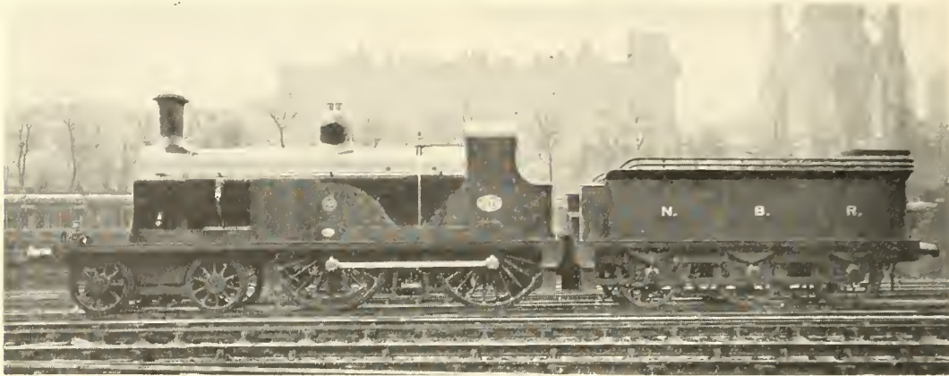
FIG. 340—M. HOLMES'S 7ft. COUPLED EXPRESS ENGINE, NORTH BRITISH RLY., 1886
