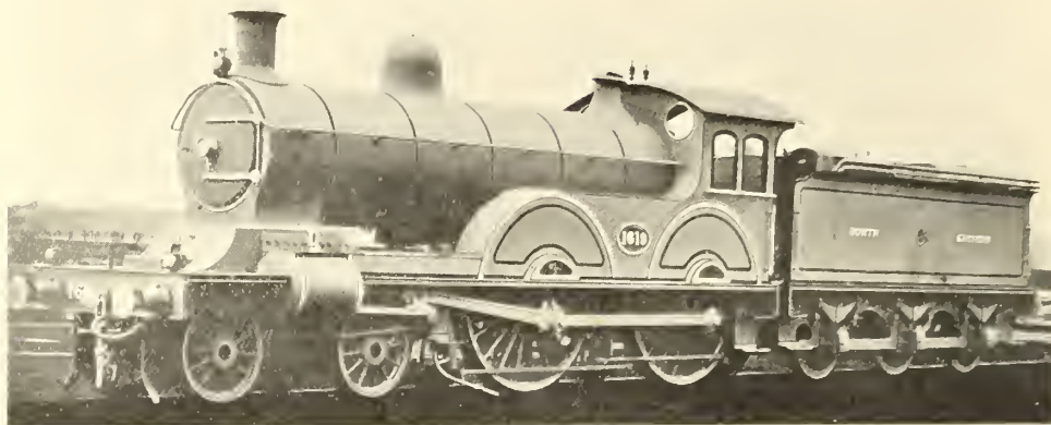
FIG. 362—W. WORSDELL'S EXPRESS ENGINE No. 1619, N.E. RLY., REBUILT AS A THREE-CYLINDER COMPOUND, 1893
