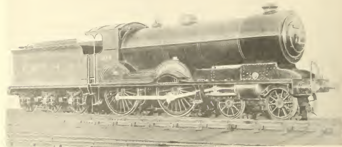
FIG. 451—FOUR CYLINDER EXPRESS ENGINE, GLASGOW & SOUTH-WESTERN RLY., REBUILT BY R. H. WHITELEGG, 1923
