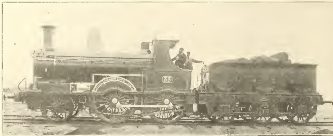
FIG. 363—B. MALCOLM'S TWO-CYLINDER COMPOUND ENGINE, BELFAST AND NORTHERN COUNTIES RLY., 1890
