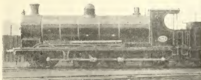
FIG. 441—J. F. McINTOSH'S EIGHT-COUPLED MINERAL ENGINE, CALEDONIAN RLY., 1901-3
