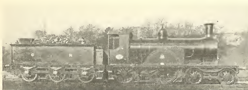
FIG. 329—NEILSON'S SINGLE DRIVER ENGINE, CALEDONIAN RLY., 1886 [Photo. Locomotive
