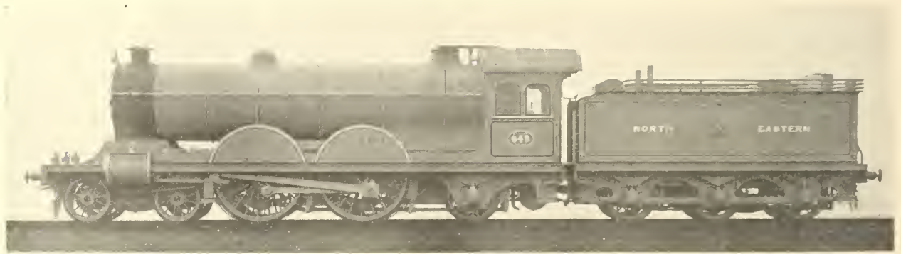
FIG. 417—W. WORSDELL'S "ATLANTIC" TYPE EXPRESS ENGINE, NORTHEASTERN RLY., 1904
