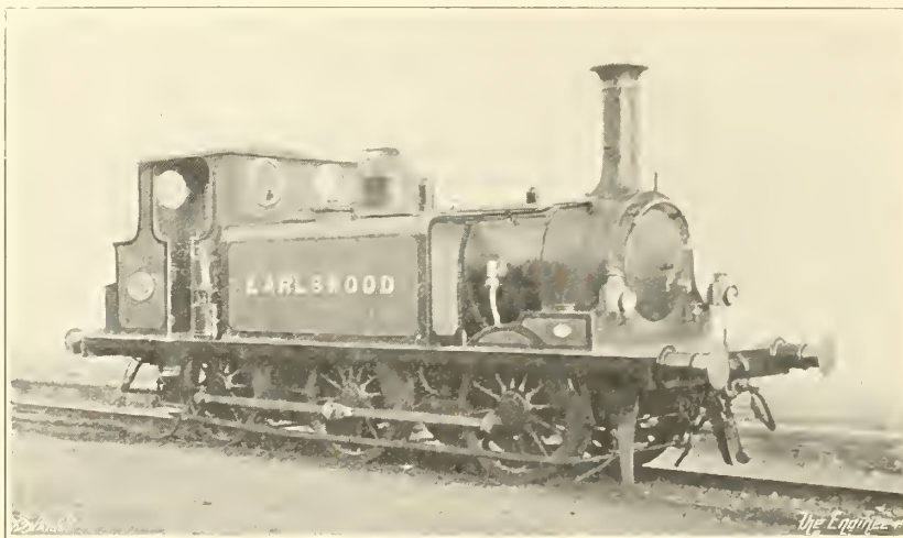
FIG. 263—W. STROUDLEY'S L.B. & S.C.R. "TERRIER" TANK ENGINE, 1872-80
