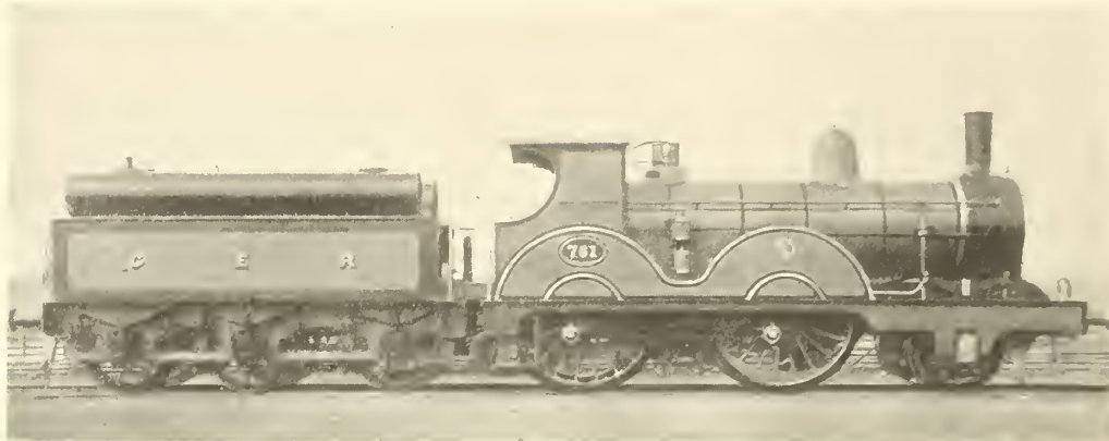
FIG. 334—J. HOLDEN'S OIL-FUEL EXPRESS ENGINE. GREAT EASTERN RLY., 1886-97
